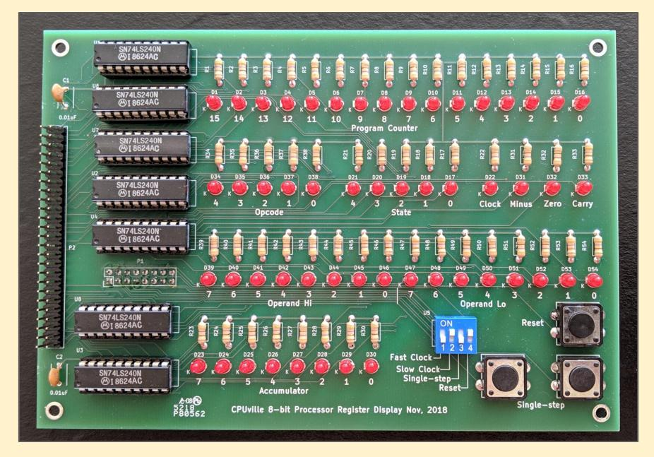
This is not a full sized set of registers! It's a register display kit to enable the workings of a CPU to be modelled
