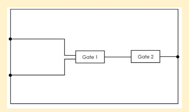
The expression **B OR (NOT A)** can be represented by the logic circuit shown below. In the circuit the logic gates are marked with labels instead of their proper symbols.
