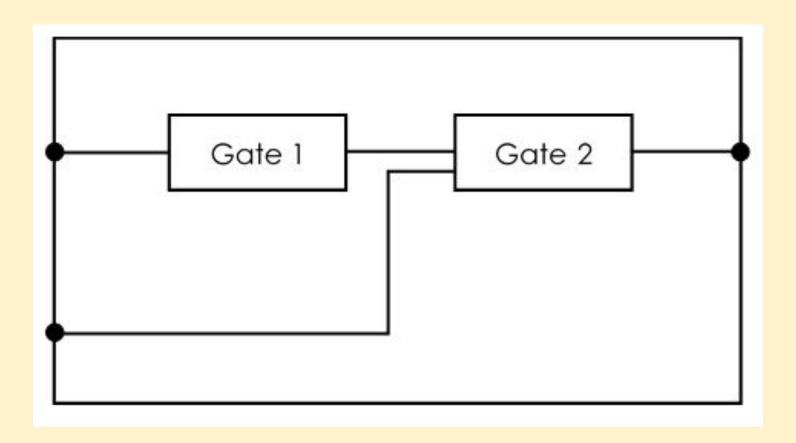
The expression (A AND B) OR (B AND C) can be represented by the logic circuit shown below. In the circuit the logic gates are marked with labels instead of their proper symbols.
